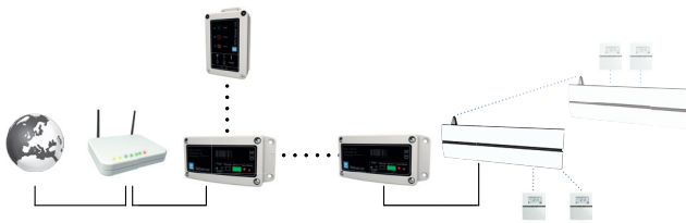
An example of a system with a webserver as a communication bridge. The webserver is connected to both the water safety system and room temperature control ICS.2.
